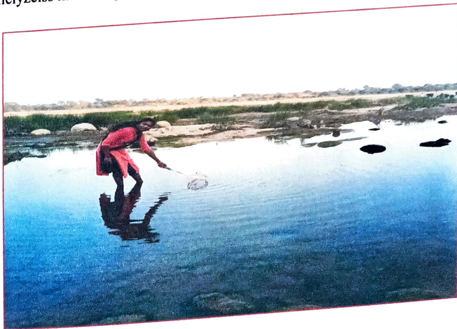
Sweeping method to collect sample
